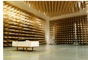
Anechoic chamber used for electromagnetic wave measurement
