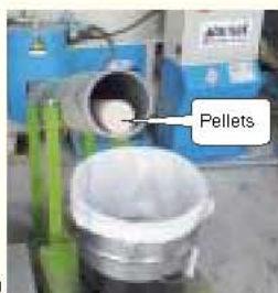
Sawdust pelletizing system (Kakegawa Factory)
