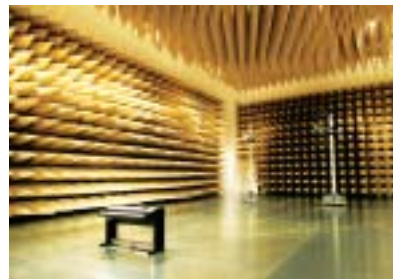
Anechoic chamber used for electromagnetic wave measurement
