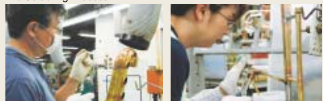
Keiji Sone (right) and Shunichi Niwata display some wind instruments in the crafts workshop of Yamaha Corporation's Toyooka Factory. Sone: "When we first began using lead-free solder, our production efficiency fell more than 20%. But within about a year, we had regained our previous level of efficiency." Niwata, holding artist model YTR-9445CHS (custom-made gold plated): "This particular trumpet was developed to reflect input from a group of top artists brought together by a member of our American R&D team. Lead-free solder was one of many specifications included from the outset."
