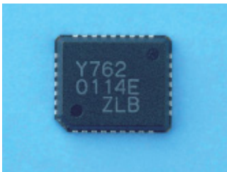
Mobile Phone Sound Chip YMU 762 ▶ These 40-note polyphony sound chips include built-in ADPCM (Adaptive Differential Pulse Code Modulation) sound generators that can play back human voices and other recorded sounds.
