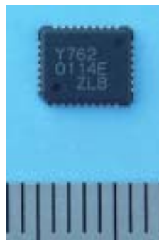
Sound Chip YMU 762 ▶ These 40-note polyphony sound chips include built-in ADPCM (Adaptive Differential Pulse Code Modulation) sound generators that can play back human voices and other recorded sounds.
