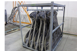
Returnable packing rack for grand piano frames
