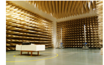
Anechoic chamber used for electromagnetic wave measurement
