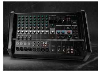
The EMX Series offers the same features as a stand-alone analog console: built-in compression, 3-channel semi-parametric EQ, and up to 24 DSP presets for effects. The EMX7 also has a 9-band EQ and an on-board feedback suppressor.
