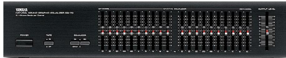
Graphic equalizers (GEQs) are used to correct the frequency response of a speaker. Connect the main outputs of your console to the GEQ and use it to “tune the room” or correct problem frequencies caused by standing waves in the room (reflections).
