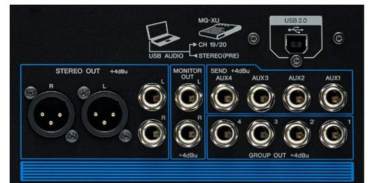
Ensure the AUX Outputs on the back of the mixing console are connected to the correct monitors and/or FX processors.
