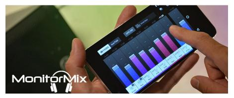
By setting up a closed Wi-Fi router and connecting it to your digital console, you can create a private network for the band to log in and create their monitor mixes. You won't be able to hear your mix through the phone — you'll still need earphones and a wired or wireless headphone amp connected into the audio system. Then, you can adjust your mix personally, on the fly, through the phone.
