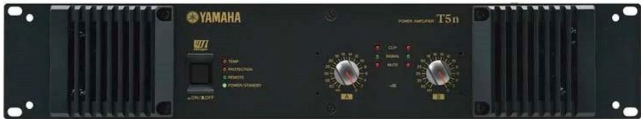
Power is measured in watts and sometimes referred to as program, continuous or root-mean-square (RMS) power rating. It's the continuous music power that the amplifier can deliver. You must use an amp that is 50% more powerful than your speakers.
