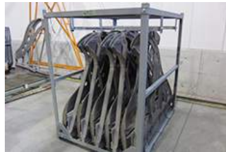
Newly-introduced returnable packing rack for GP frames
