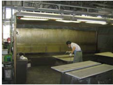
Wet painting booth(Kakegawa Factory)
