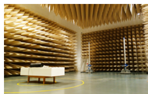
Anechoic chamber used for electromagnetic wave measurement
