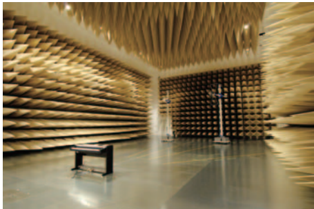
Anechoic chamber used for electromagnetic wave measurement
