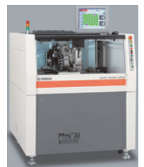
“Micro-prober” Conduction break inspection machine
