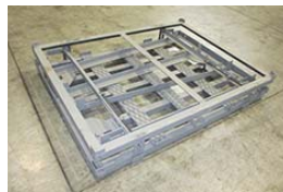
Folded packing rack (when being returned)
