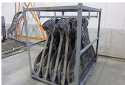
Returnable rack for grand piano frames
