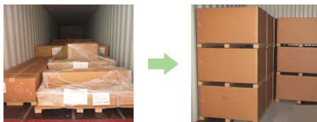
Loading container with packing boxes prior to standardization (left), Loading container using standardized packing boxes (right)
