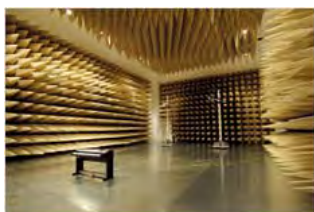
An anechoic chamber used for electromagnetic wave measurement
