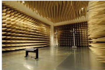
Anechoic chamber used for electromagnetic wave measurement
