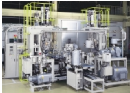
YAMAHA's AW-30 aluminum wheel leakage-inspection system for automobiles
