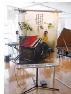
Thin (1mm), light (400g/m 2 ) and flexible TLF speakers can be produced in large sheets and printed on the surface.
